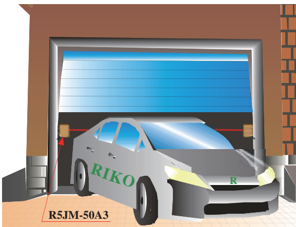
Detecting if the car drive out of garage. 車庫車輛進出確認
